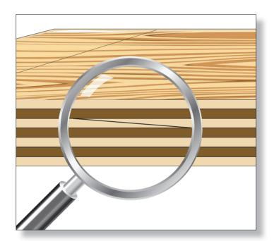
**SCARFING:** End to end joining of veneer. Makes a long piece of veneer from short pieces. The joint is an 8:1 slope, bonded with exterior glue, and APA approved.
